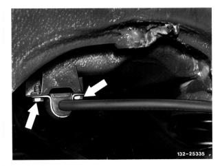
32.0701 - 310/2 32 .07.01 - 340/ B 2 4 Loosen propeller shaft intermediate bearing.
